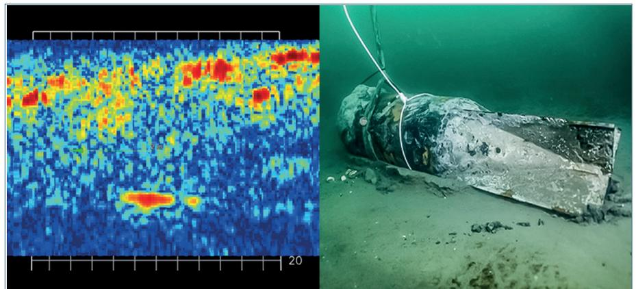
Figure 2: The SBI image of the buried target (left), identified as an elongated, elliptical target lying parallel to the seabed and the recovered UXO (right)
