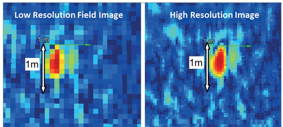
Figure 3: Standard 10cm voxel SBI data (left) and a 5cm rendered example of the same anomaly (right), enhancing the shape of anomalies in 3D acoustics
