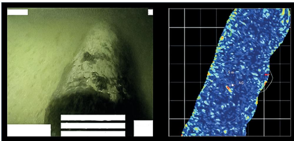
Figure 5: Recovered UXO (left) and the 3D acoustic image (right) demonstrating good correlation to the as-found anomaly
