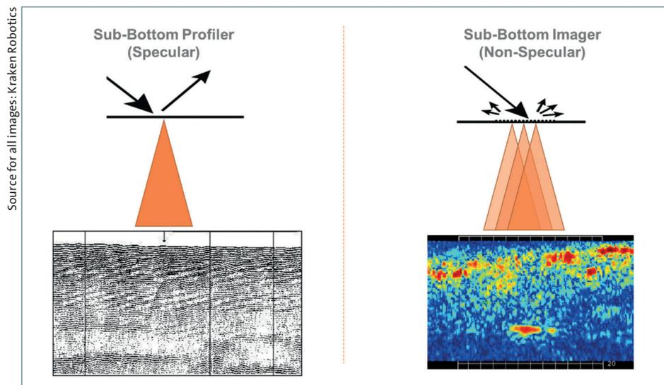
Figure 1: Aspecular acoustic return typical of a sub-bottom profile (left), and the SBI's non-specular acoustic return imaging the targets exterior (right)
