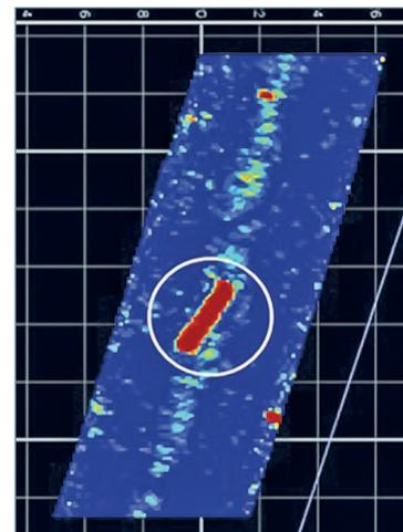
Figure 6: A very clear acoustic image of a non-ferrous UXO
