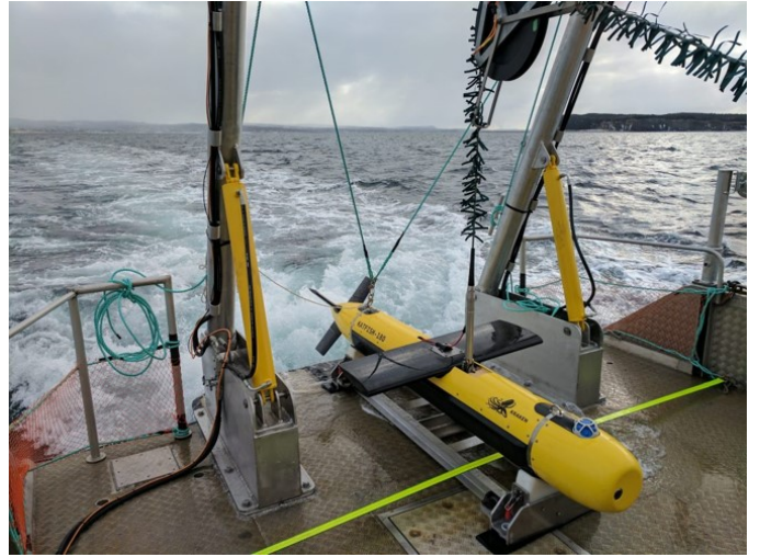
Fig. 1. KATFISH™ actively controlled towfish with AquaPix® Miniature Interferometric Synthetic Aperture Sonar (MINSAS).
