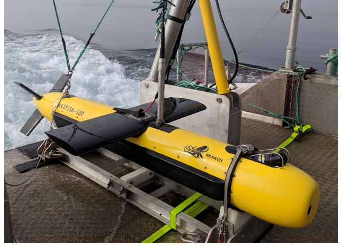
Fig. 2. KATFISH, Kraken's actively controlled towfish, equipped with the MINSAS180.
