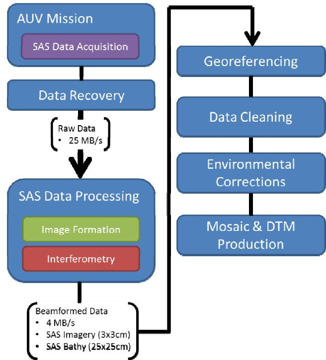
**Figure 3: Typical SAS Data Processing Stages**
