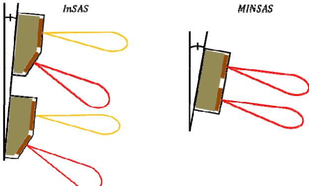
**Figure 10: InSAS vs. MINSAS Transducer Design**
