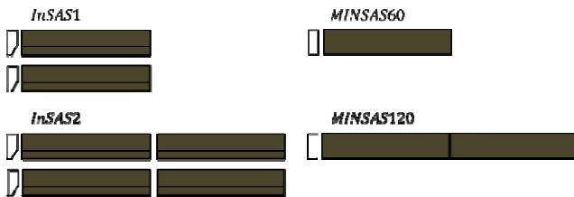
**Figure 12: InSAS vs. MINSAS Transducer Configuration**
