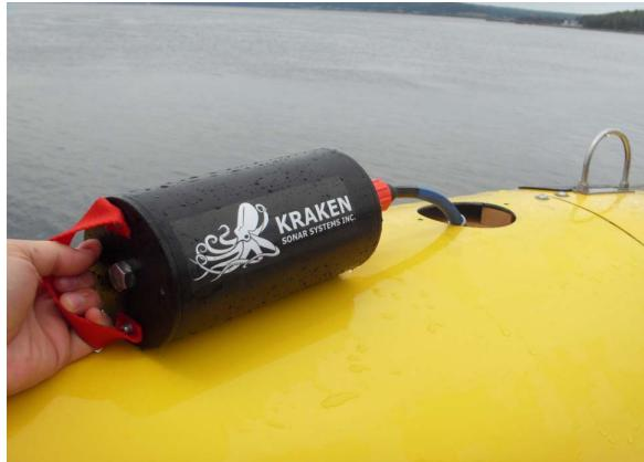
**Figure 7: Kraken DataPod Removed from an AUV**
