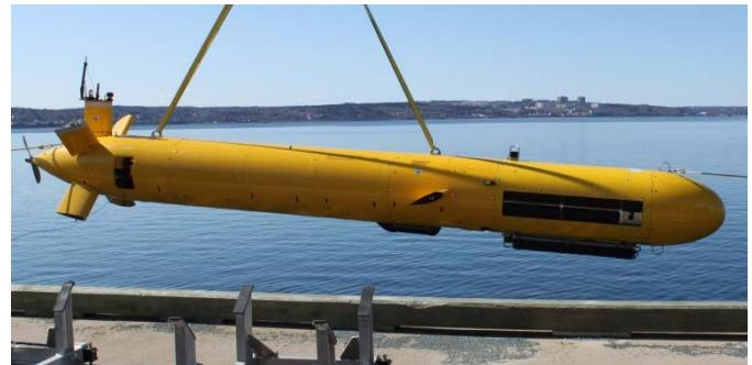
**Figure 14: DRDC Arctic Explorer with InSAS2 and MINSAS120**
