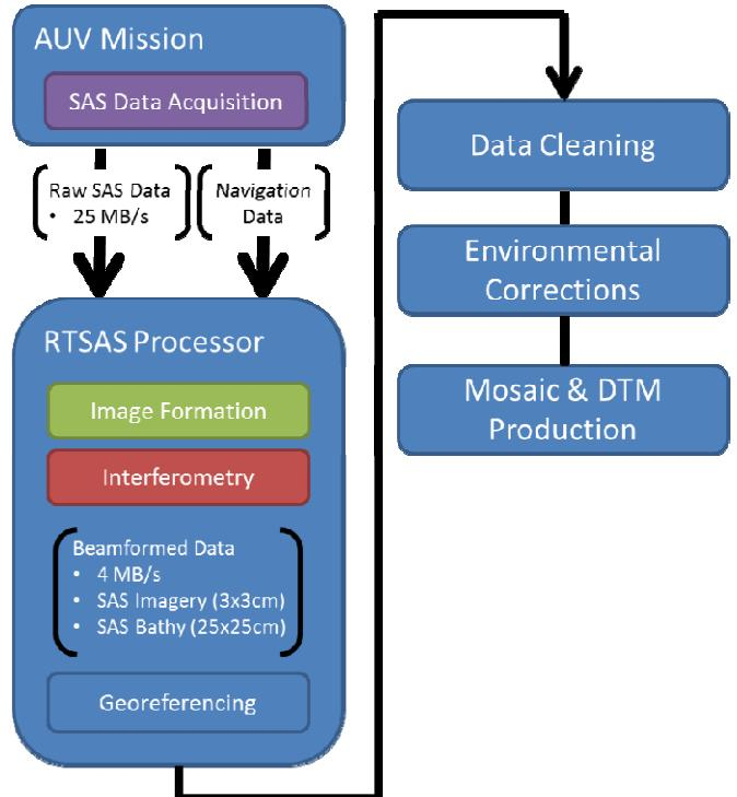
**Figure 6: SAS Data Workflow with RTSAS Processor**
