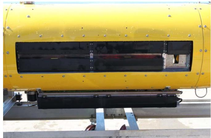
**Figure 13: MINSAS120 Installed Below InSAS2**
