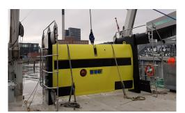
SeaKite allows high-speed SBI data collection up to 4 knots in waters up to 250 meters depth. This remotely operated towed vehicle (ROTV) can be utilized on a smaller vessel with smaller crew size compared to traditional ROV surveys.
