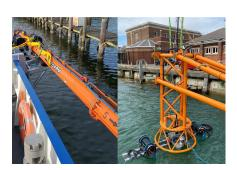
For nearshore applications, the SBI GeoArm and GeoLink can be mounted to vessels and operate in shallow waters up to 15 meters depth in areas such as ports, rivers, and nearshore environments.
