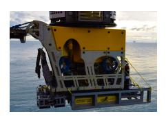
The SBI can be deployed from 3 to 500 meters on multiple platforms for all your survey requirements. The SBI ROV mount can be adapted to fit all work-class ROVs with custom skids available to fit lighter ROVs.
