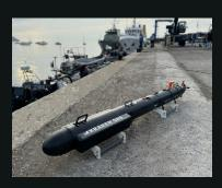
Kraken's light-weight man-portable synthetic aperture sonar (MP-SAS) brings increased capability to low logistics, small class UUV surveys. Kraken MP-SAS uses Kraken SAS technology as a foundation, with modifications to reduce size, weight, and power.
