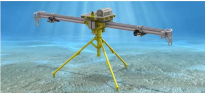
Fig. 1. Acoustic Corer with a tripod leg deployed on seabed.
