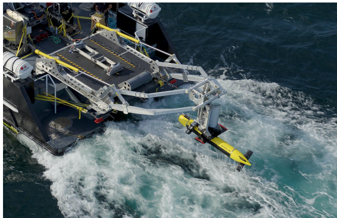
Fig. 1. R/V Ocean Seeker with Kraken’s SeaScout system consisting of a launch and recovery system, KATFISH actively controlled towfish, and AquaPix Miniature Interferometric Synthetic Aperture Sonar (MINSAS).
