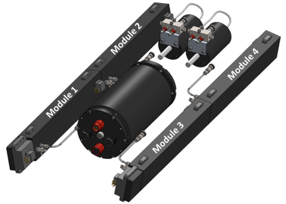
Fig. 1. AquaPix® Miniature Synthetic Aperture Sonar (MINSAS) with modular receiver array (four receiver modules and two transmitter modules shown), electronics pressure vessel (large cylinder), and port and starboard oil compensation units (small cylinders).
